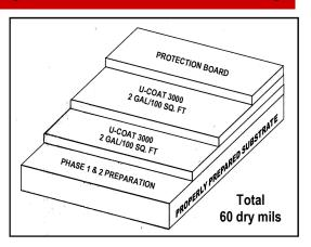
**Phase 4:** The second coat of U-Coat 3000 should be applied at a rate of 2 gallons/100 sq. ft.  $(0.82 \text{ liters/m}^2)$  resulting in a 30  $\pm$  2 dry mils  $(762 \pm 51 \text{ microns})$  membrane. At 75°F  $(24^{\circ}\text{C})$  and 50% relative humidity, allow a minimum of 24 hours before checking watertightness.
